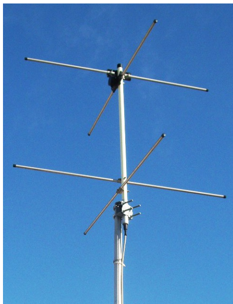
Figure 2.4: Example of an omnidirectional antenna.
