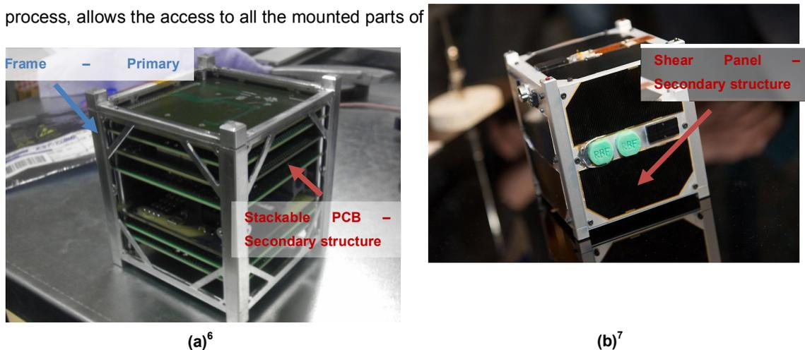
Figure 3 - CubeSat internal mounted structure (a) and external assembled structure (b)
