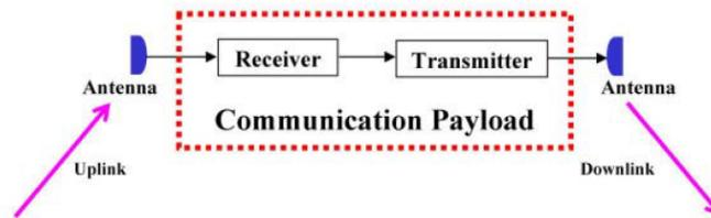
Figure 4 – Space segment COM Simplified Schematic Diagram
