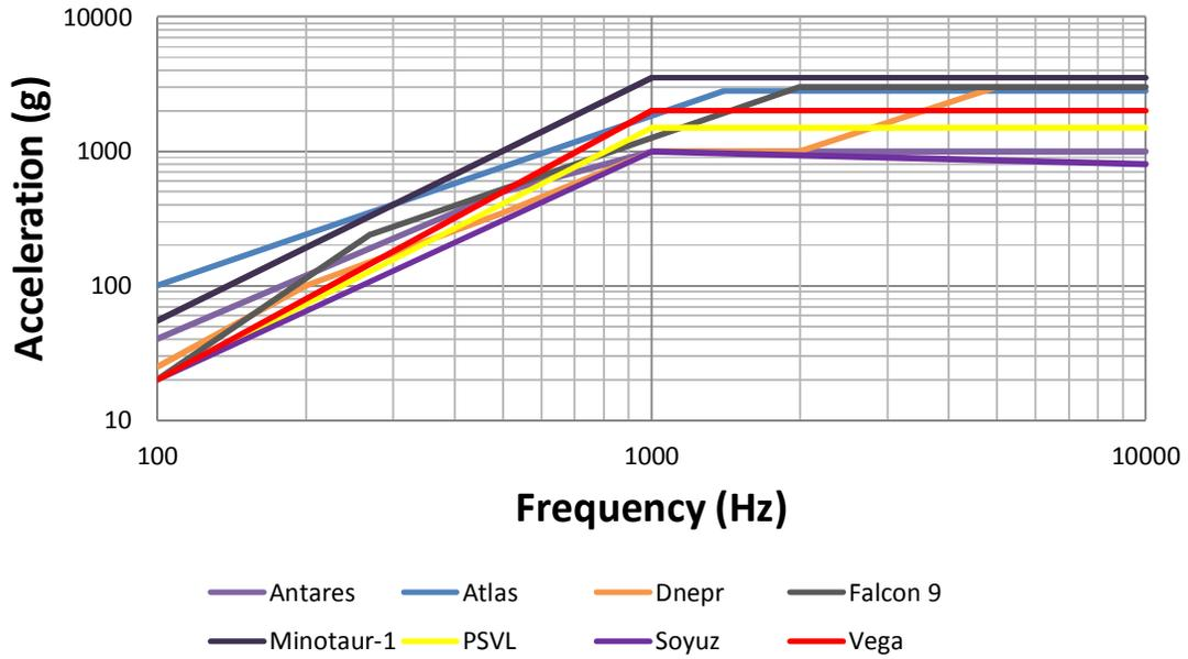
Figure 17 - Shock loads of selected launchers
