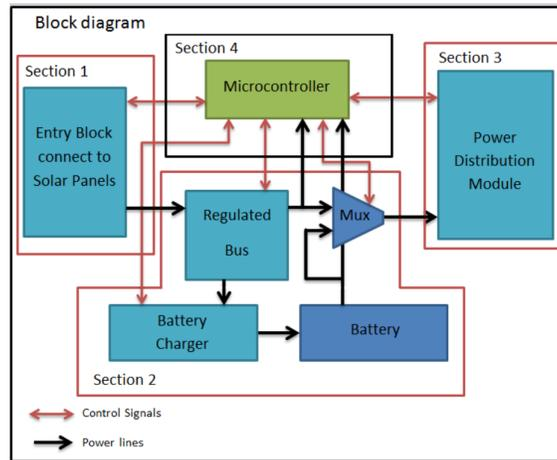
Figure 29 – EPS global architecture block [82]
