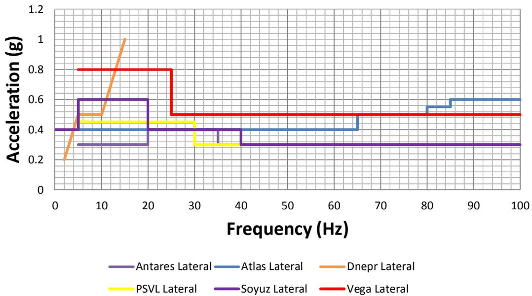
Figure 14 - Sine Equivalent Vibration Lateral loads of selected launchers
