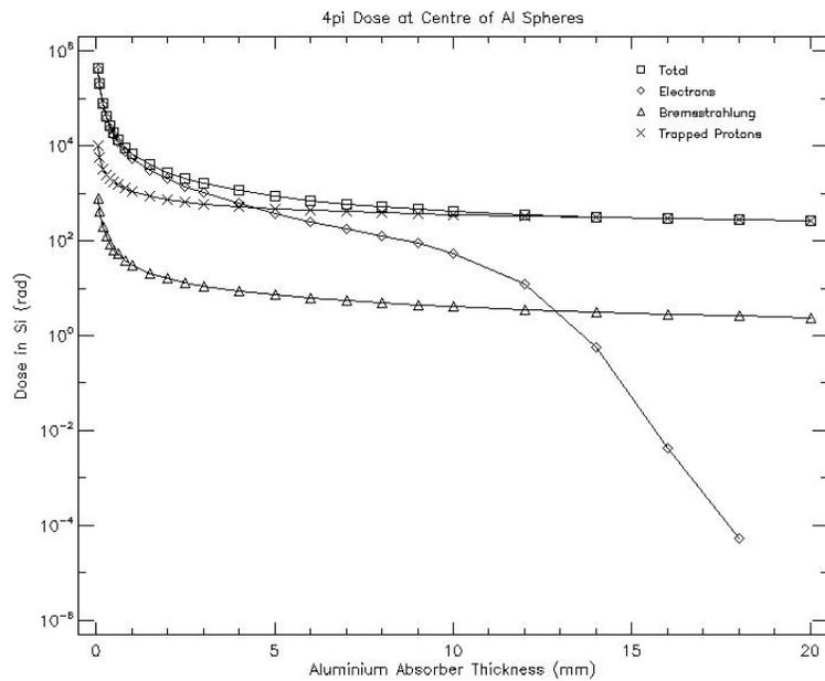
Figure 22 – Radiation levels for a 1-year circular orbit R=1000 Km per Al shielding thickness
