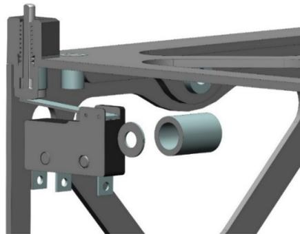
Figure 28 – ISTNanosat-1 power switch mechanism
