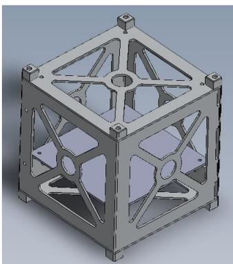
Figure 26 – ISTNanosat-1 structure 3D
