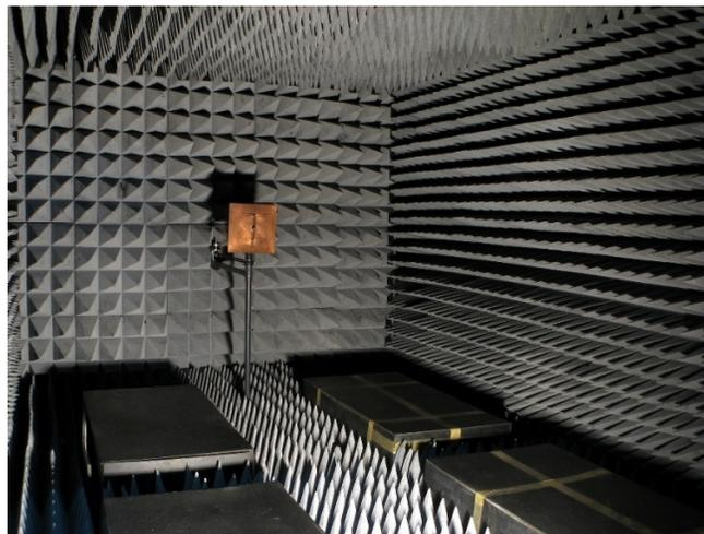
Figure 46 – Anechoic chamber example for EMC testing<sup>42</sup>
