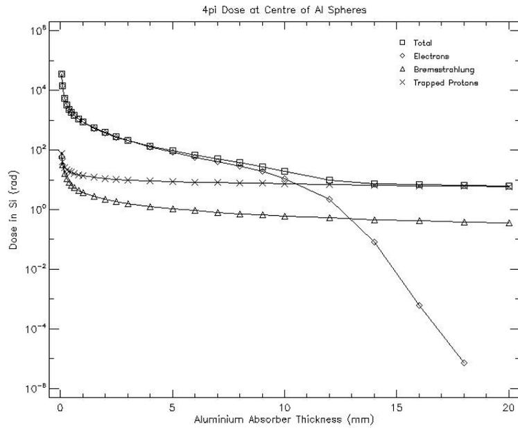
Figure 21 – Radiation levels for a 4 months circular orbit R= 400Km per Al shielding thickness
