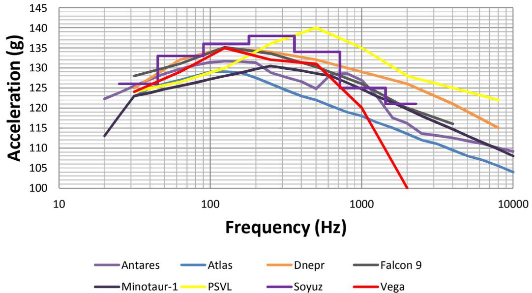
Figure 16 - Acoustic Vibration loads of selected launchers
