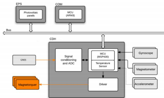
Figure 30 – Joint Board ESP+CDH architecture
