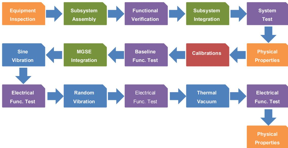
Figure 36 - PFM Detailed Test Flow
