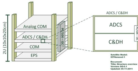
Figure 27 - ISTNanosat-1 internal structure overview
