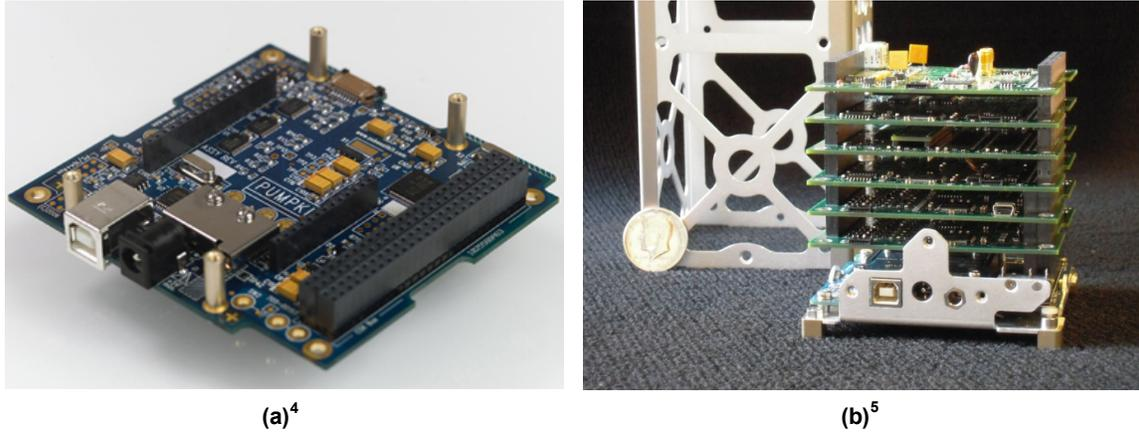
Figure 2 - PC/104 PCB (a) and CubeSat internal stacks (b)
