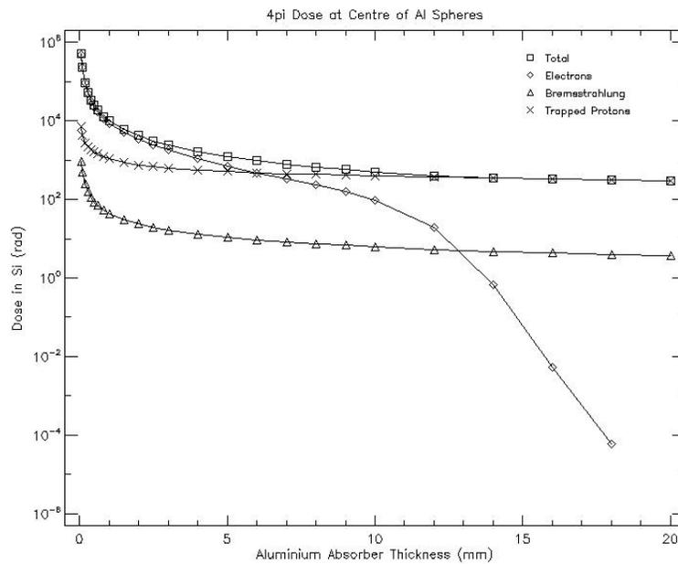
Figure 24 – Radiation levels for a 1-year polar orbit AP=10000 Km per Al shielding thickness
