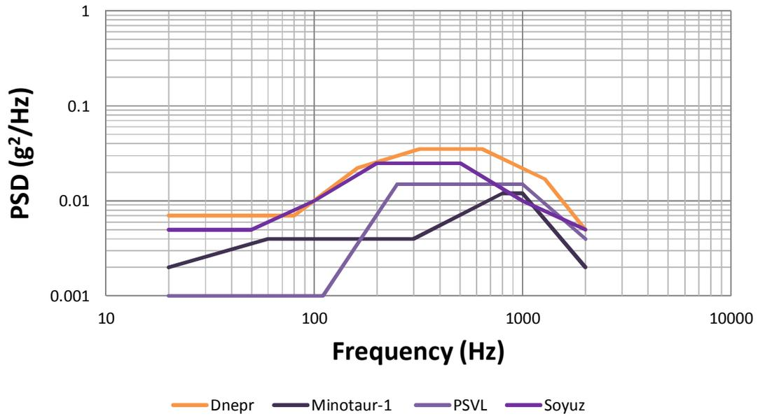
Figure 15 - Random Vibration loads of selected launchers
