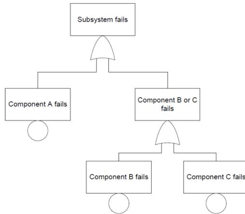
Figure 9 - Sample fault tree diagram [62]
