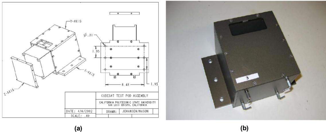
Figure 34 – CubeSat Test POD schematics (a) and Test POD (b) [84]
