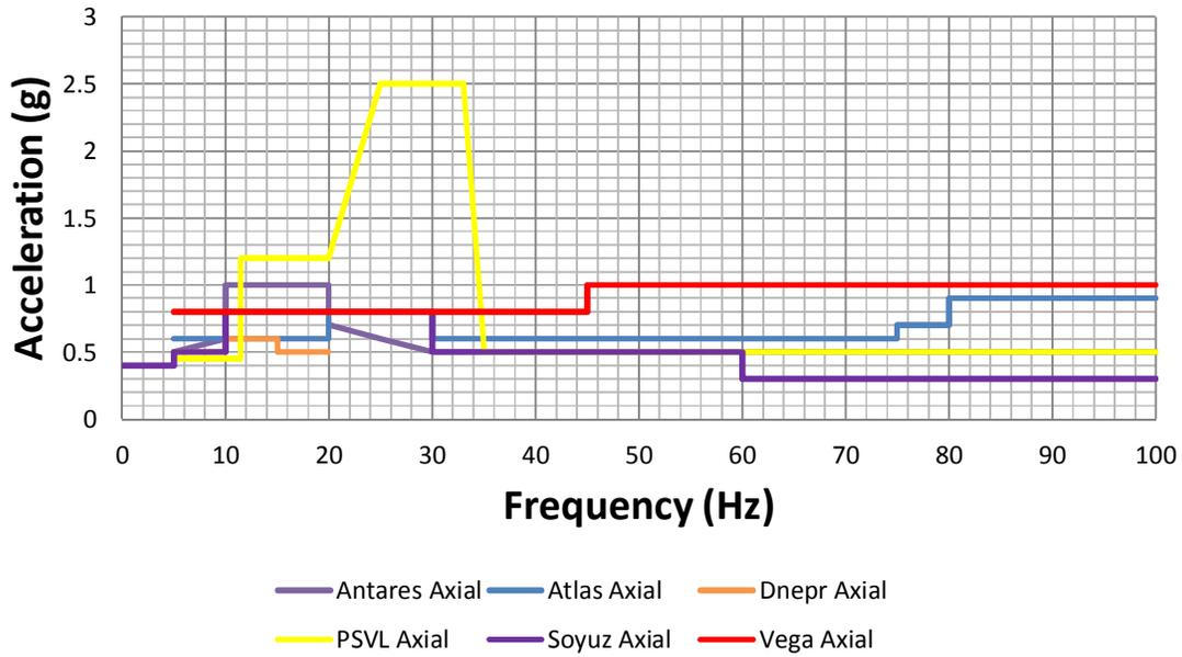
Figure 13 - Sine Equivalent Vibration Axial loads of selected launchers
