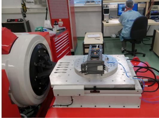
Figure 39 – Vibration Shaker example<sup>39</sup>
