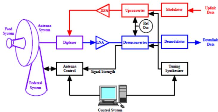
Figure 6 - Typical summarized ground station architecture [52]
