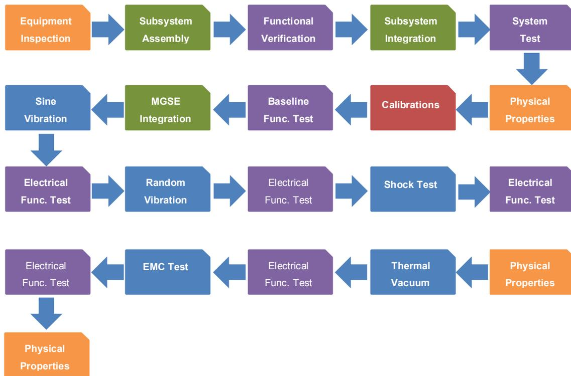
Figure 37 – EQM Detailed Test Flow
