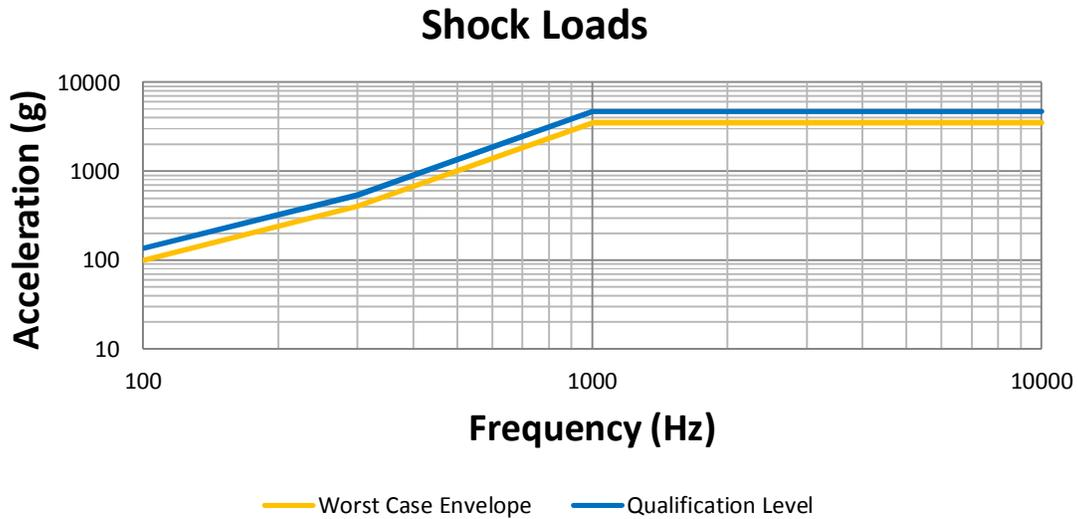
Figure 43 – Mechanical Shock Qualification Test Level
