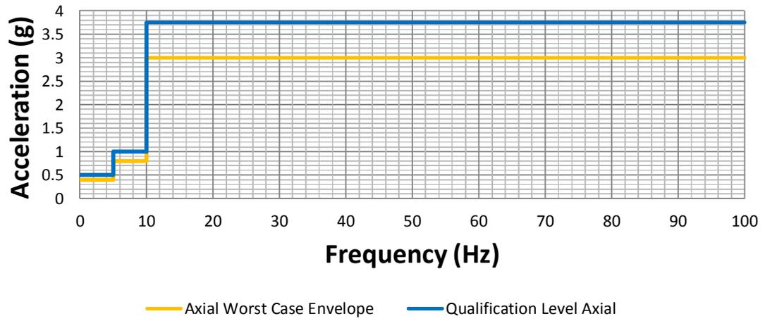
Figure 40 – Sine vibration Qualification Test Level
