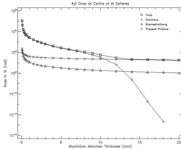
Figure 20 – Radiation levels for a 1-year circular orbit R=400 Km per Al shielding thickness
