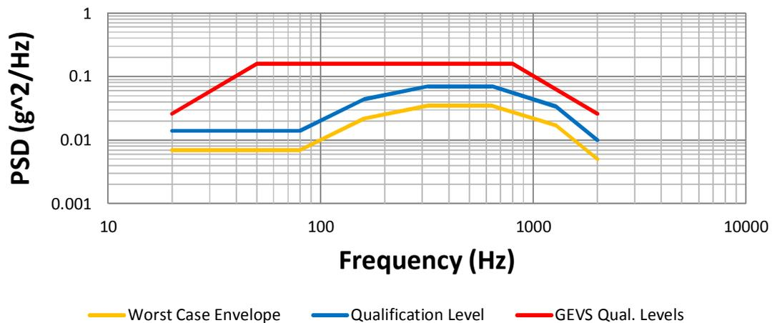
Figure 41 - Random Vibration Qualification Test Level
