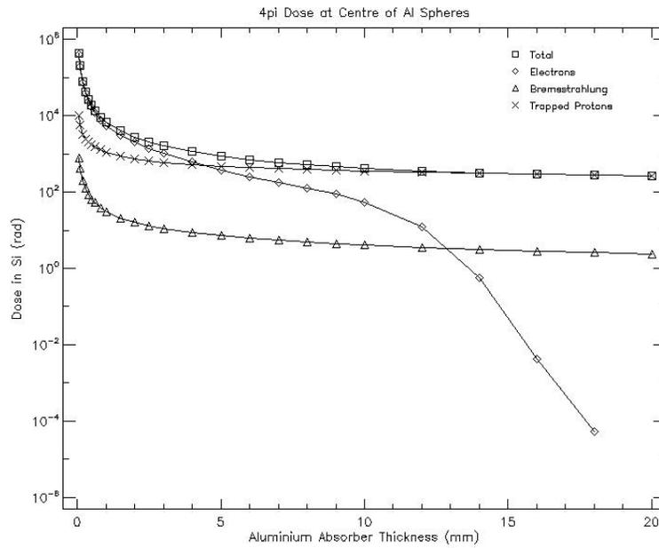
Figure 23 – Radiation levels for a 4 months circular orbit R=1000 Km per Al shielding thickness
