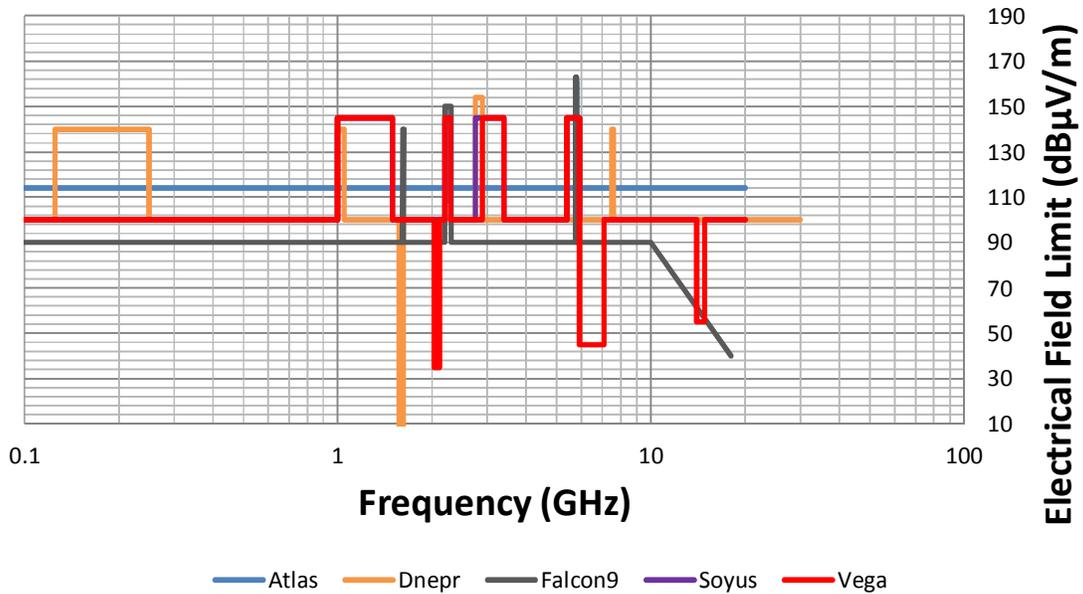
Figure 18 – Worst Case Electromagnetic Environment of selected launchers
