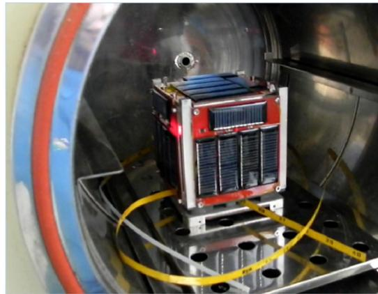
Figure 44 – Thermal Vacuum Chamber example<sup>41</sup>
