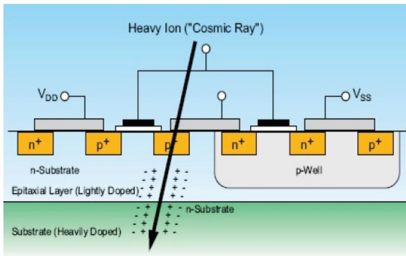
Figure 25 – Single Event Effect illustration on EEE<sup>34</sup>
