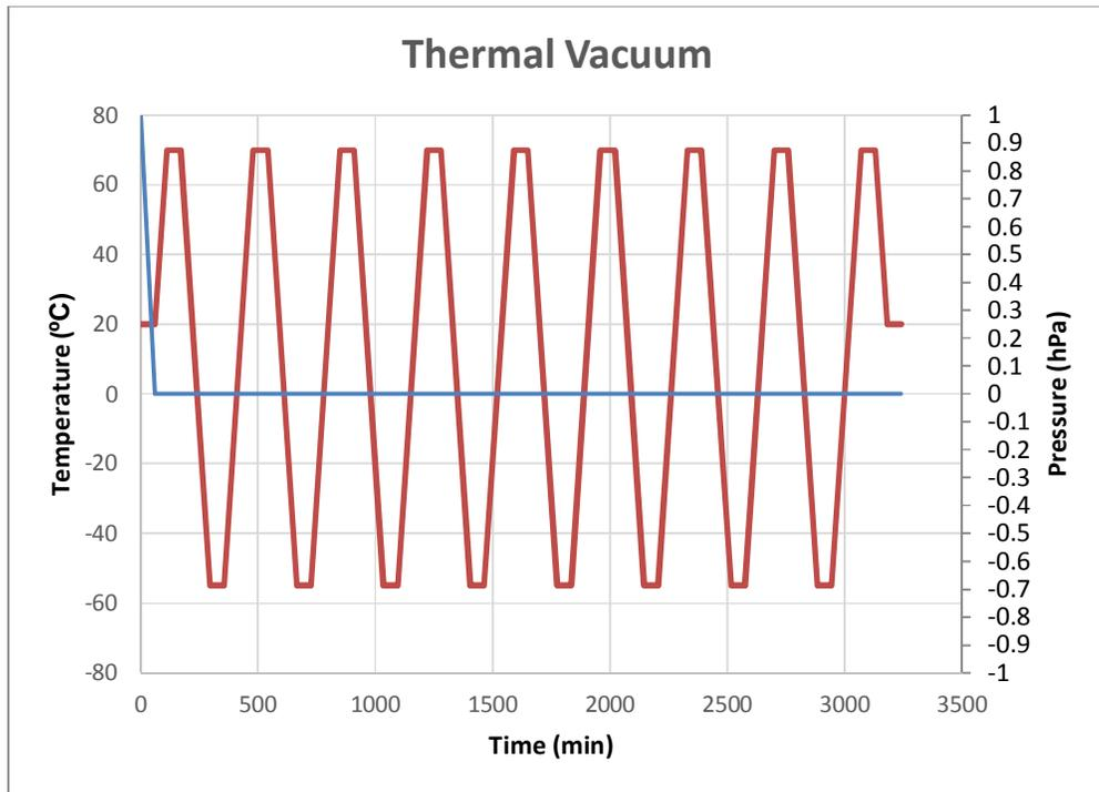
Figure 45 - Thermal Vacuum test levels
